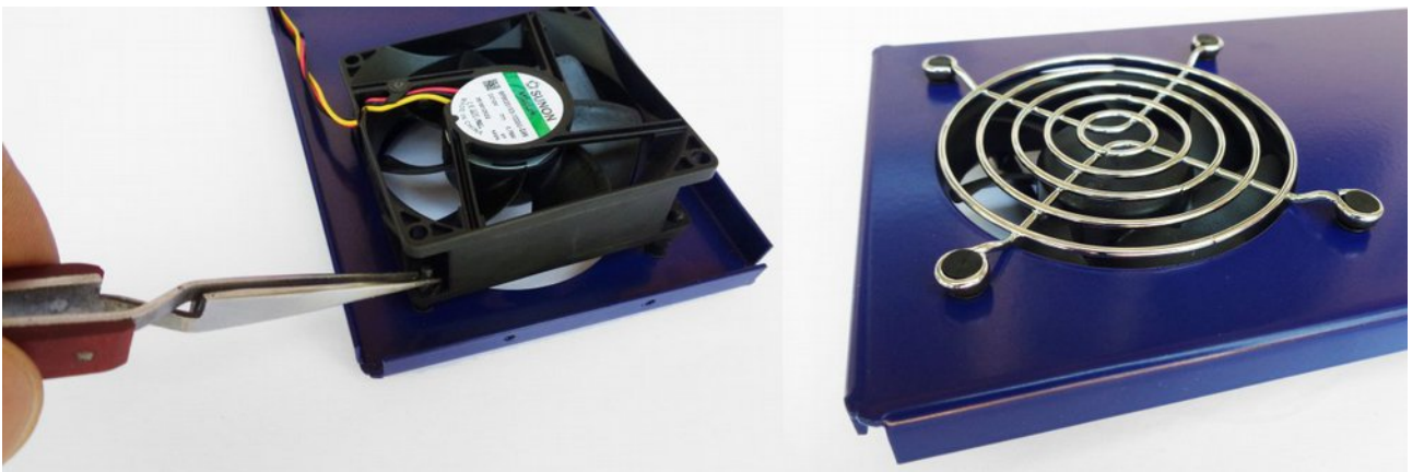
Fig. 9: Mounting fan and finger guard
